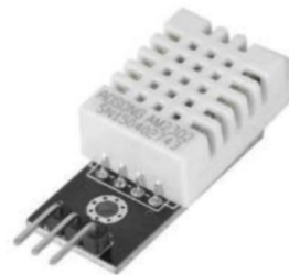
Fig. 3. DHT22 temperature and humidity sensor.
