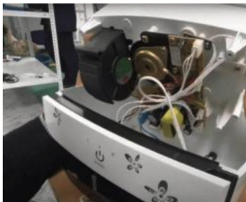
Fig. 4. Humidifier construction from inside.
