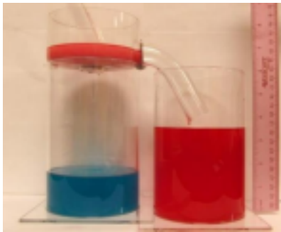
Figure 2 - A new type of filter separates water (blue) from oil (red).
